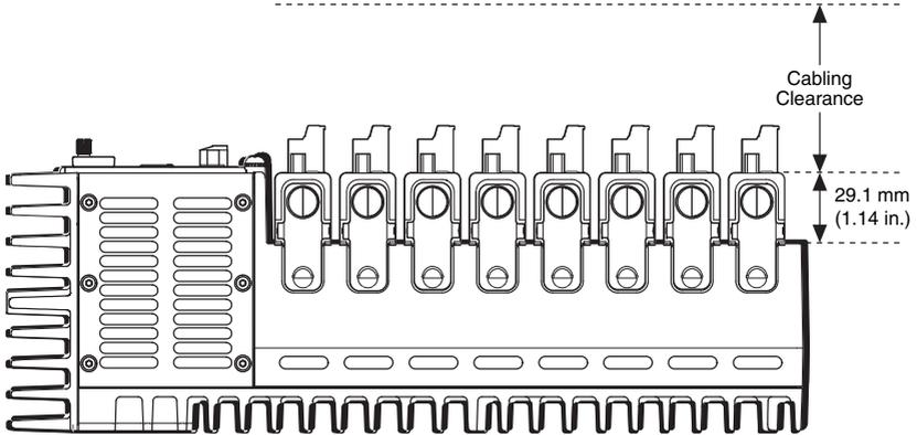
Measure the ambient temperature at each side of the cRIO-904x, 63.5 mm (2.50 in.) from the side and 38.1 mm (1.50 in.) forward from the rear of the cRIO-904x, as shown in the following figure.
