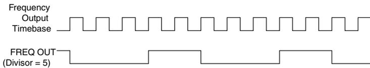
Frequency Output can be routed out to any PFI terminal. All PFI terminals are set to high-impedance at startup. The FREQ OUT signal also can be routed to many internal timing signals.
