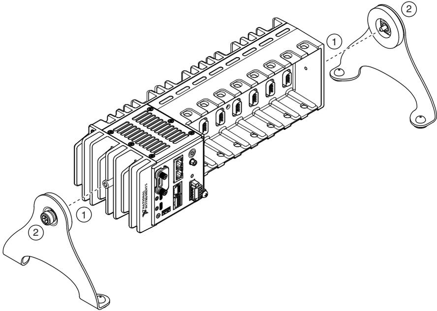
1. Align the brackets with the mounting holes on the ends of the cRIO-904x.
