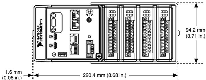
**Figure 10.** 8-slot cRIO-904x Module Immobilization Accessory Dimensions
