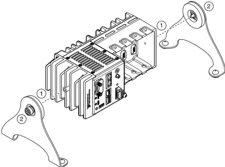
**Figure 30.** Mounting the 8-slot cRIO-904x on a Desktop
