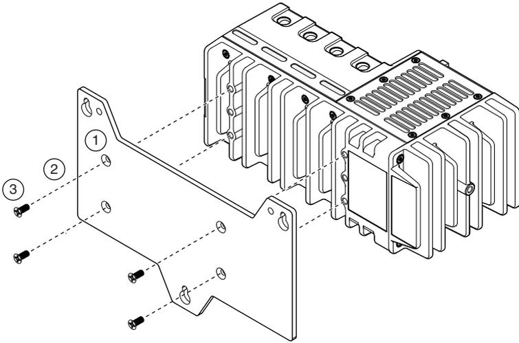
**Figure 23.** Mounting the 8-slot cRIO-904x on a Panel
