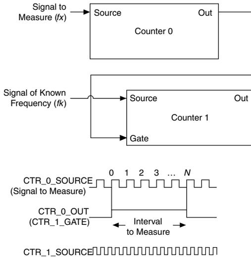
Next, route the Counter 0 Internal Output signal to the Gate input of Counter 1. You can route a signal of known frequency ( $f_k$ ) to the Counter 1 Source input. Configure Counter 1 to perform a single pulse-width measurement. Suppose the result is that the pulse width is  $J$  periods of the  $f_k$  clock.
