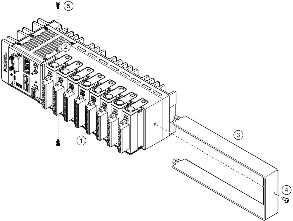
1. Ensure that all the C Series modules are installed in the cRIO-904x and the latches are locked in place.
