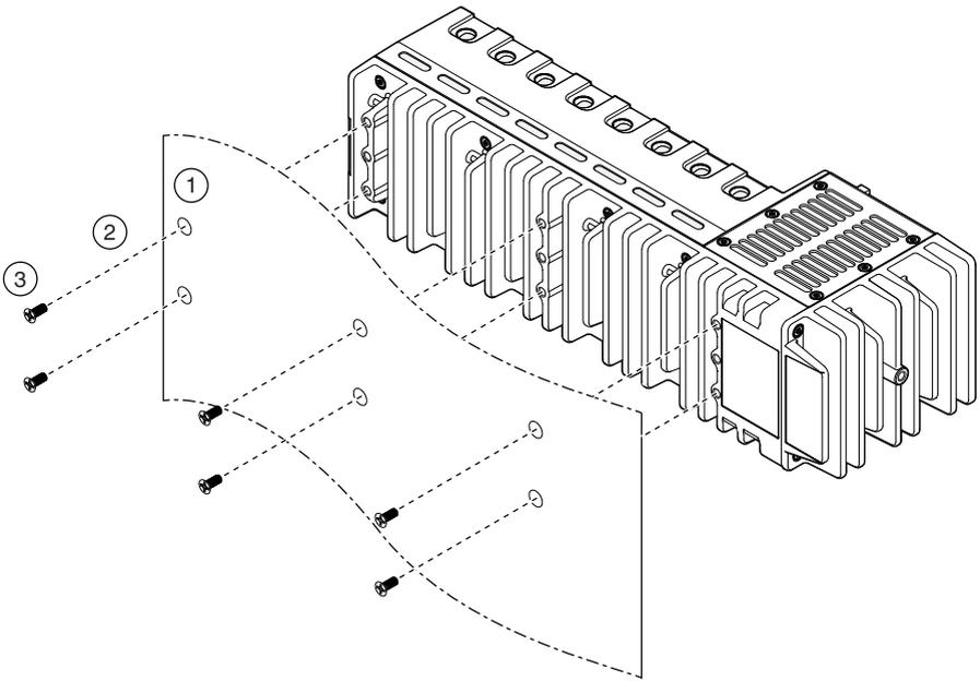
1. Prepare the surface for mounting the cRIO-904x using the [Surface Mounting Dimensions](#).
