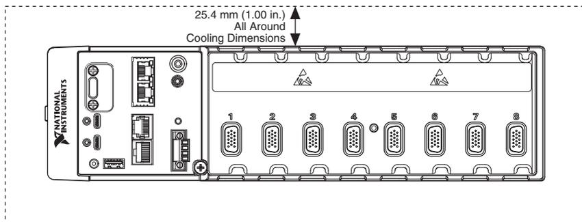
Allow the appropriate space in front of C Series modules for cabling clearance, as shown in the following figure. The different connector types on C Series modules require different cabling clearances. For a complete list of cabling clearances for C Series modules, visit [ni.com/info](http://ni.com/info) and enter the Info Code `crioconn`.
