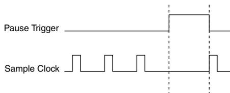
If you are using any signal other than the onboard clock as the source of the sample clock, the generation resumes as soon as the pause trigger is deasserted and another edge of the sample clock is received, as shown in the following figure.
