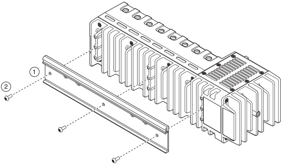
1. Align the cRIO-904x and the DIN rail clip.
