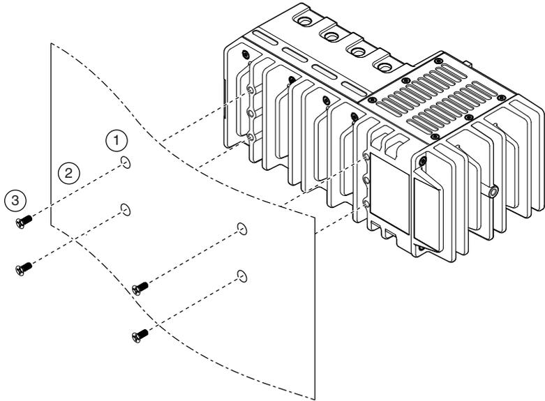
**Figure 19. Mounting the 8-slot cRIO-904x Directly on a Flat Surface**
