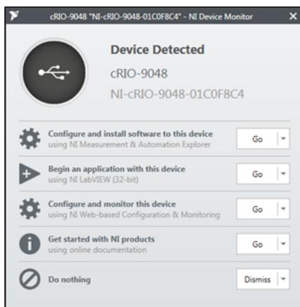
If the device driver software does not detect the cRIO-904x, verify that you installed the appropriate NI software in the correct order on the host computer as described in "Installing Software on the Host Computer" in the *cRIO-904x Getting Started Guide*.
