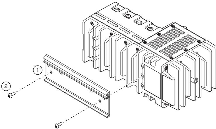
**Figure 27.** Mounting the 8-slot cRIO-904x on a DIN Rail
