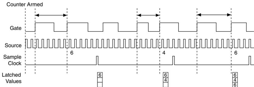
With sample clocked frequency measurements, ensure that the frequency to measure is twice as fast as the sample clock to prevent a measurement overflow.
