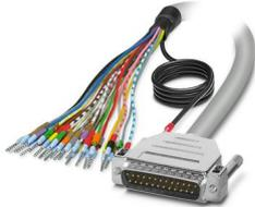
Assembled shielded round cable; connection 1: Single wires (25-position) (The wires are marked and fitted with ferrules. The braided shield is routed to a separate cable end.); connection 2: D-SUB pin strip (1x 25-position); cable length: 1 m
