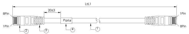
INK MARKING<FP2049>: CAT.6 S/FTP PATCH CABLE 3P VERIFIED TO ANSI/TIA-568.2-D ▲ 26AWGX4P VW-1(UL)
