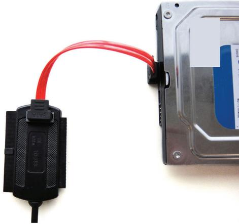
(2) Have the external Power Adapter connect with USB 2.0 TO IDE/SATA ADAPTER CABLE.
