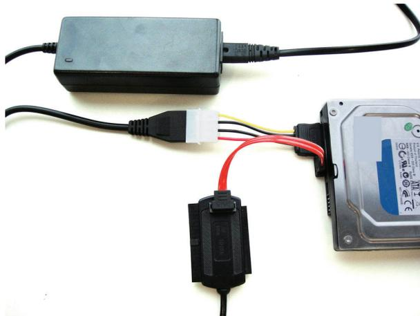
(3) Have USB 2.0 TO IDE/SATA ADAPTER CABLE connect with and your computer, then power on, your computer system will detect the SATA HDD.
