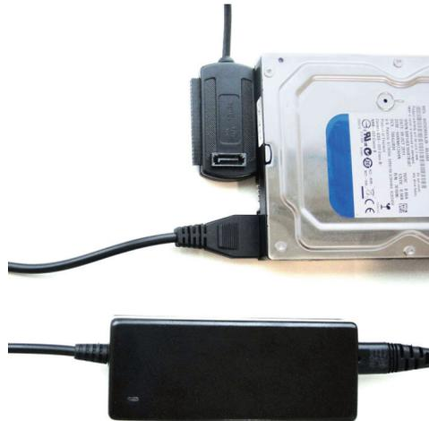
(3) Have USB 2.0 TO IDE/SATA ADAPTER CABLE connect with your computer, then power on, your computer system will detect the IDE HDD.
