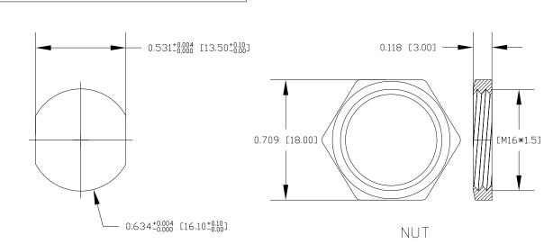
NOTE: MATERIAL HOUSING: PBT UL94V-0, BLACK CONTACT: BRASS NUT: BRASS SHELL: BRASS □-RING: EPDM, BLACK FINISH CONTACT: GOLD PLATED, 10 µ" Min. UNDER PLATE: NICKEL NICKEL PLATED NUT: SHELL: NICKEL PLATED ELECTRICAL RATED CURRENT: 4 A RATED VOLTAGE: 250V 100Μ $\Omega$  MIN INSULATION RESISTANCE: CONTACT RESISTANCE:  $10m\Omega$  MAX WATER PROOF: IP67/68 ENVIRONMENT OPERATION TEMPERATURE: -40°C ~ +85°C
