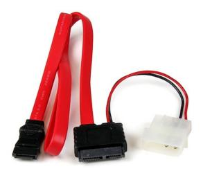
The SLSATAF36 Slimline SATA to SATA with LP4 Power Cable (36-inch) features a SATA data receptacle and a LP4 power connection on one end, and a Slimline Serial ATA receptacle on the other - allowing you to connect a slim SATA drive to a computer motherboard that does not have a Slimline connection available.
