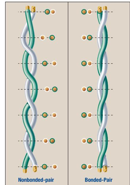
Installed and manipulated nonbonded-pairs (left) have a tendency to gap, varying the centricity of the two conductors. Belden Bonded-Pairs (right) do not gap so the physical integrity of the pair is maintained.
