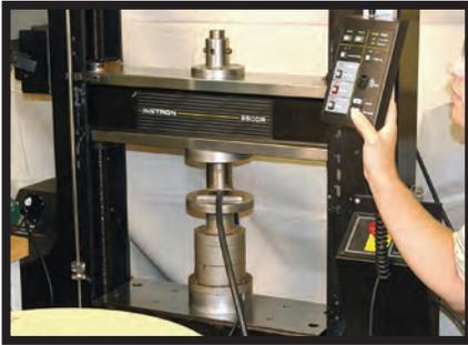
The Instron crushing device.
