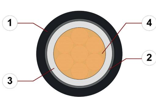
1. Outer jacket: Pressure extruded, halogen-free TPE mixture
