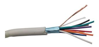
These 24AWG (American Wire Gauge) 9 bare copper conductor RS-232 multiconductor cables are used to create serial patch cables for a wide variety of applications, usually for computer peripherals.
