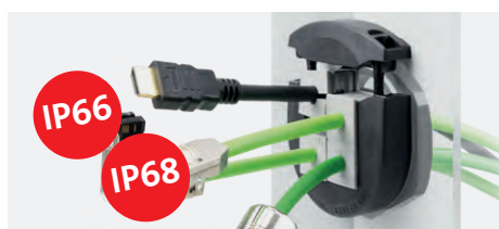
Split cable glands M25 – M63, for cable diameters up to 35 mm
