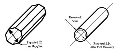
Typical applications are where tubing must fit over a large object such as in the repair or replacement of cable jacketing.
