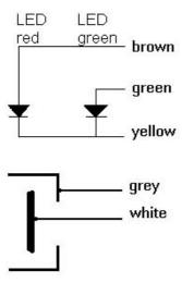
**Important**: Providing power source value higher than maximum value of  $V_F$  voltage (2,5 V for  $I_F$  = 20 mA) specified for LED is <u>not</u> recommended. If required – use the appropriate resistors for each type of LED.
