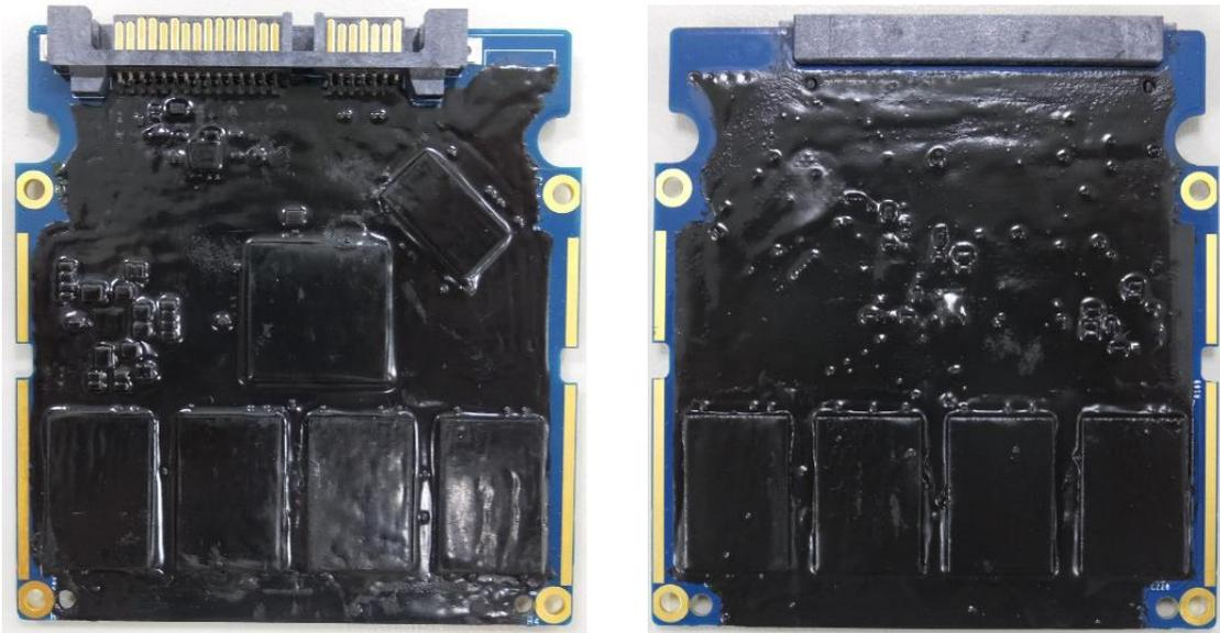
**Exhibit 2** - Specification of the 2.5-inch SATA NAND Flash SSD Cryptographic Boundary (From left to right: top side, bottom side).
