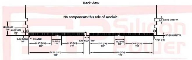
Notes: 1. All dimensions are in millimeters (inches); MAX/MIN or typical (TYP) where noted.
