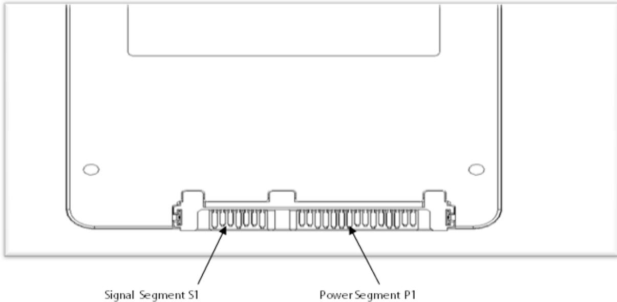
**Note:** 2.5-inch connector supports built in latching capability.
