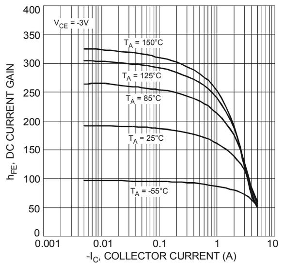
Figure 3 Typical DC Current Gain vs. Collector Current
