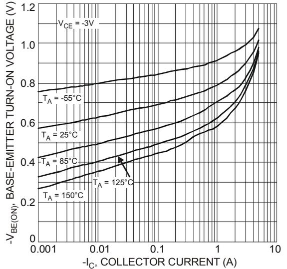
Figure 5 Typical Base-Emitter Turn-On Voltage vs. Collector Current
