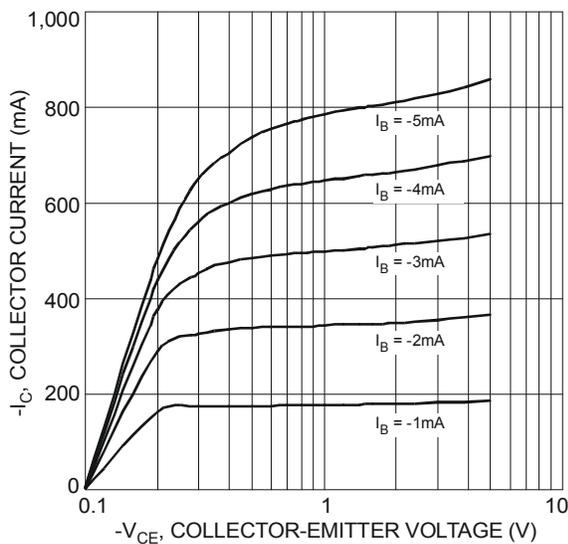
Figure 2 Typical Collector Current vs. Collector-Emitter Voltage
