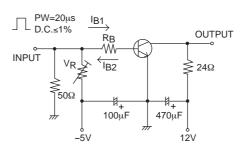
I<sub>C</sub>=20I<sub>B1</sub>= -20I<sub>B2</sub>=500mA (For PNP, the polarity is reversed)
