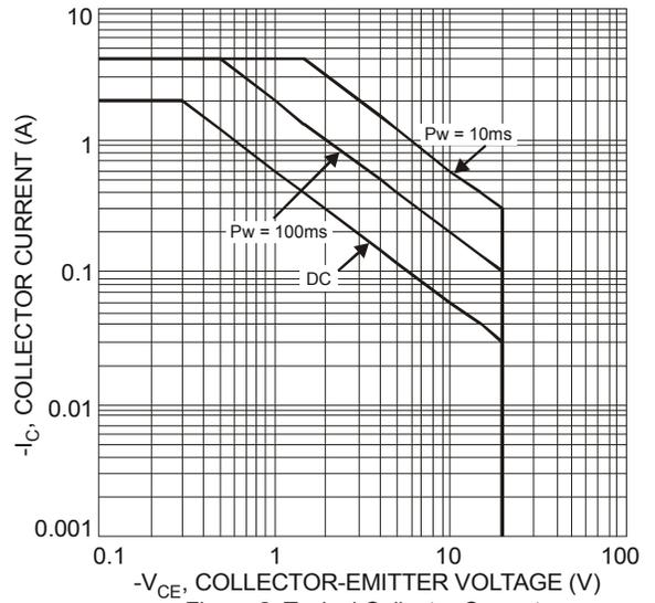
Figure 2 Typical Collector Current vs. Collector-Emitter Voltage
