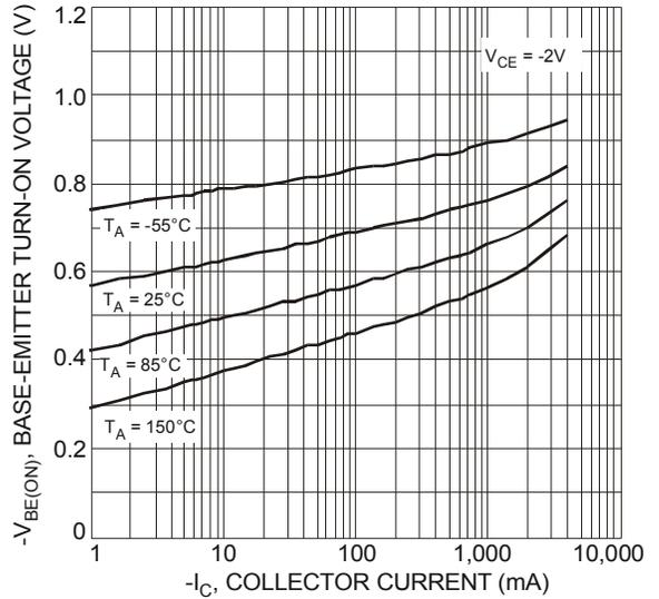
Figure 7 Typical Base-Emitter Turn-On Voltage vs. Collector Current
