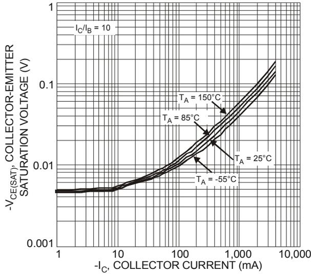
Figure 6 Typical Collector-Emitter Saturation Voltage vs. Collector Current
