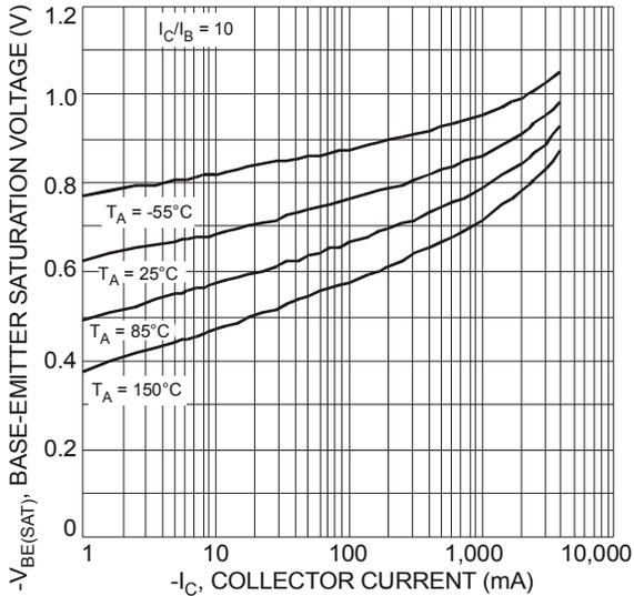
Figure 8 Typical Base-Emitter Saturation Voltage vs. Collector Current
