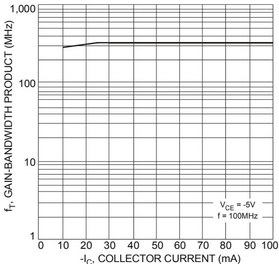
Figure 10 Typical Gain-Bandwidth Product vs. Collector Current
