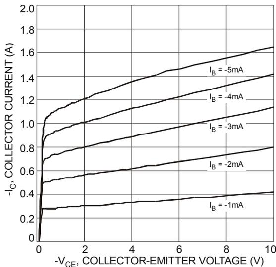
Figure 4 Typical Collector Current vs. Collector-Emitter Voltage
