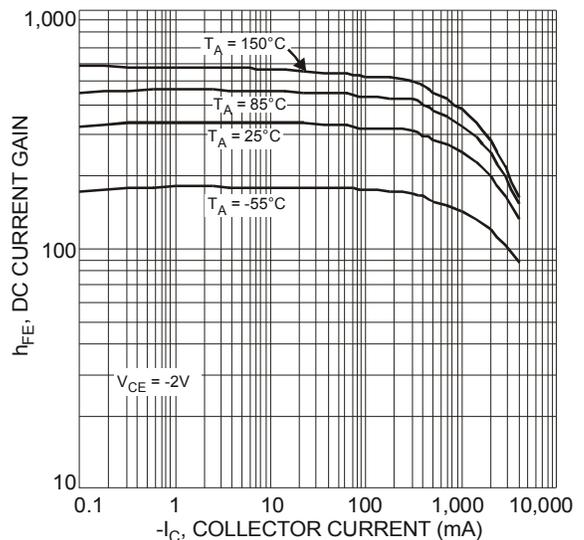
Figure 5 Typical DC Current Gain vs. Collector Current
