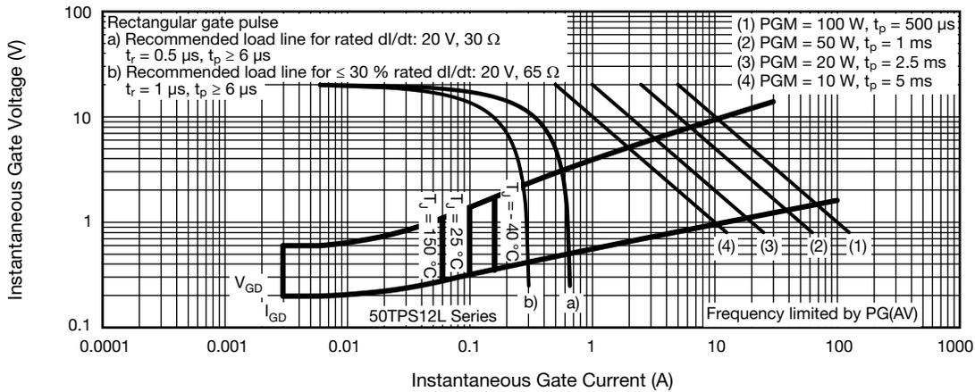
Fig. 8 - Gate Characteristics
