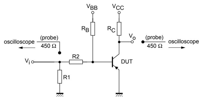
$V_i = -9.5 \text{ V}$ ,  $T = 500 \mu\text{s}$ ,  $t_p = 10 \mu\text{s}$ ,  $t_r = t_f \leq 3 \text{ ns}$ .
