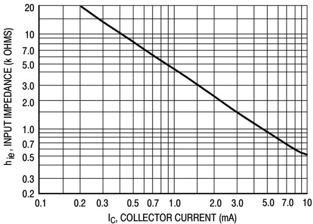
Figure 7. Input Impedance
