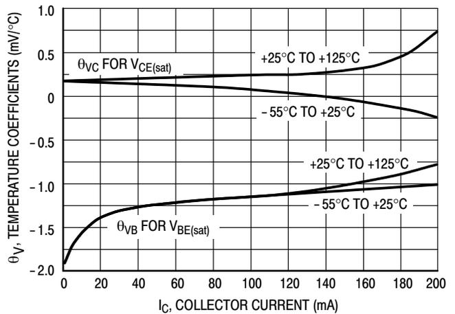
Figure 12. Temperature Coefficients
