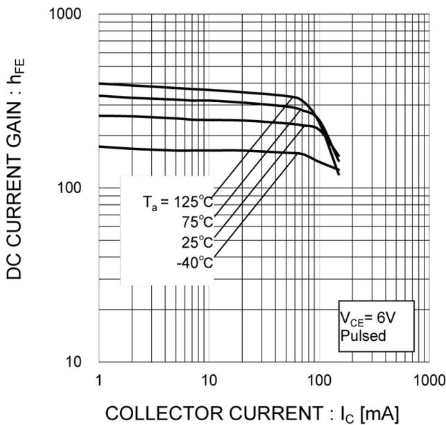
Fig.4 DC Current Gain vs. Collector Current (II)
