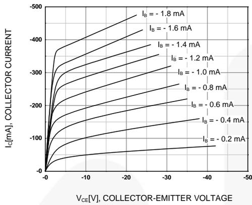
Figure 1. Static Characteristic
