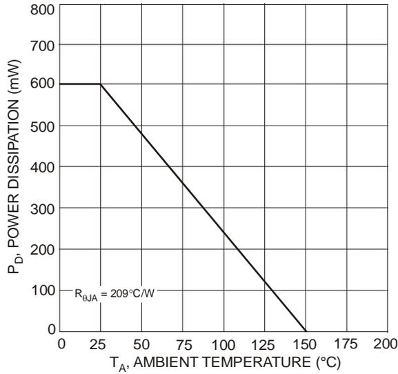
Fig. 1 Power Dissipation vs. Ambient Temperature (Note 1)
