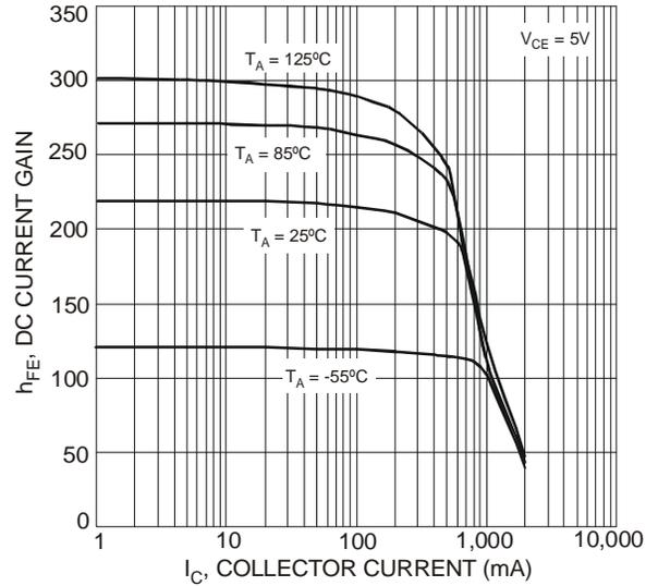
Fig. 2 DC Current Gain vs. Collector Current
