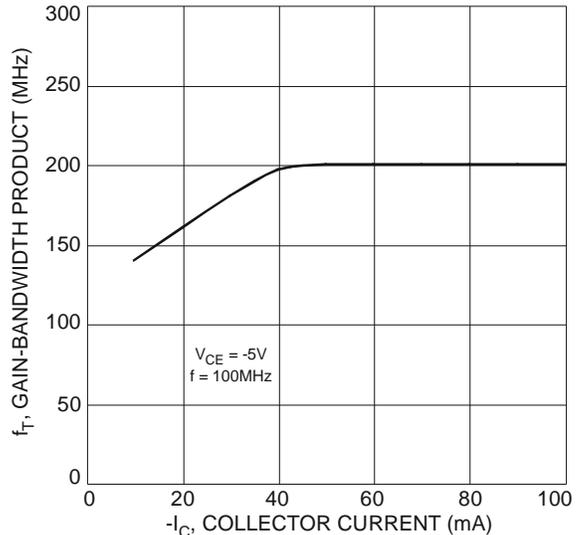
Fig. 6 Typical Gain-Bandwidth Product vs. Collector Current
