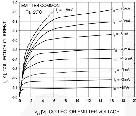
**Figure 1. Static Characteristic**
