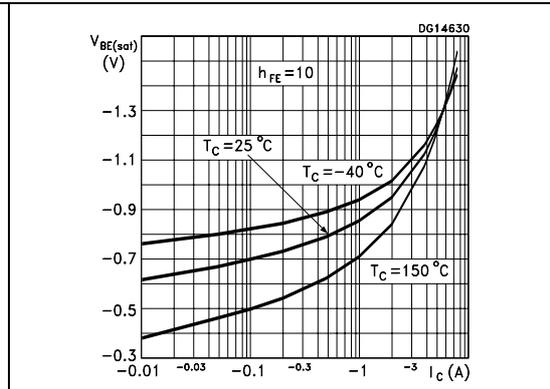
**Figure 10. Base-emitter voltage (NPN)**
