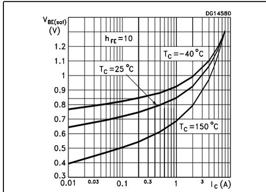
**Figure 9. Base-emitter saturation voltage (PNP)**
