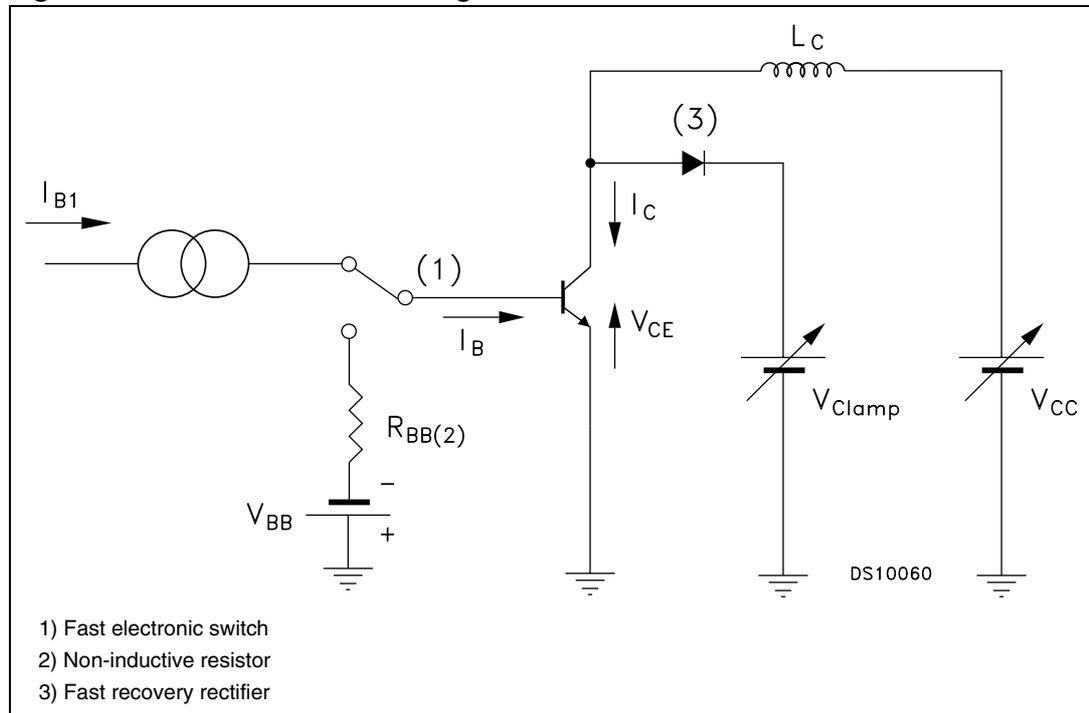
Figure 19. Resistive load switching test circuit
