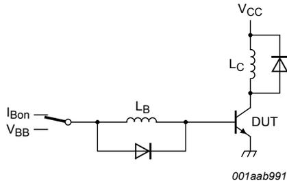
**Fig. 14. Test circuit for inductive load switching**
