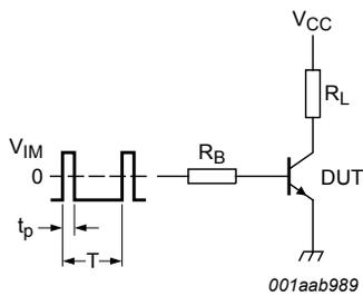
Fig. 12. Test circuit for resistive load switching
