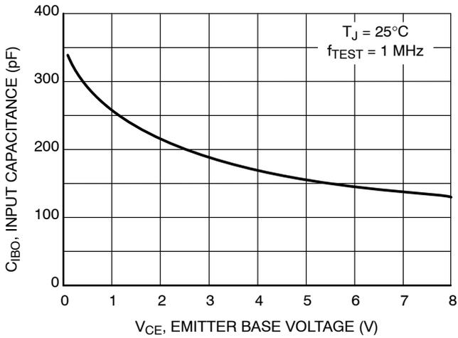
**Figure 10. Input Capacitance**
