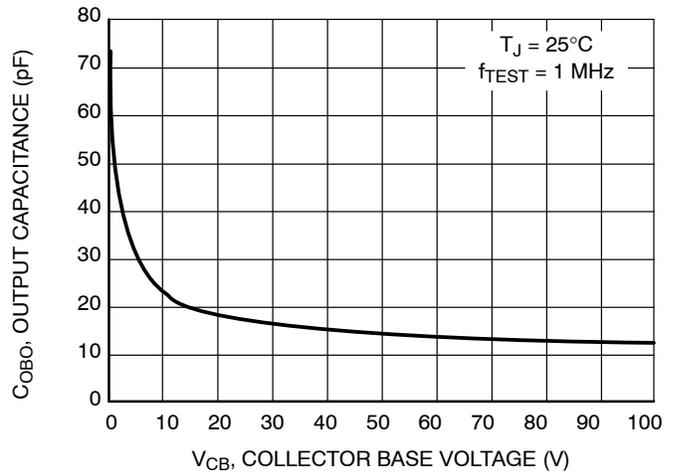
**Figure 11. Output Capacitance**
