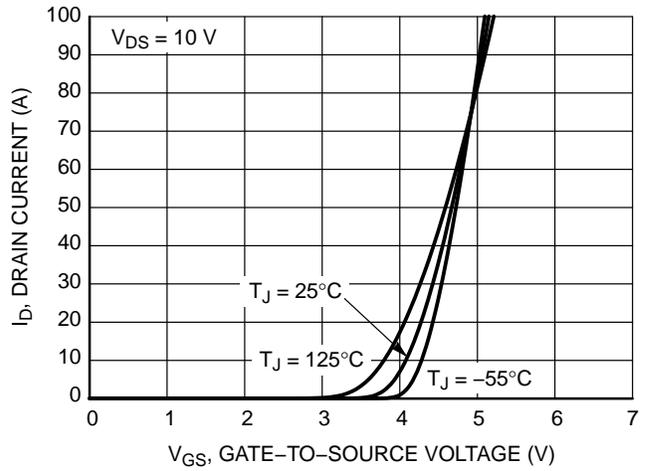
Figure 2. Transfer Characteristics
