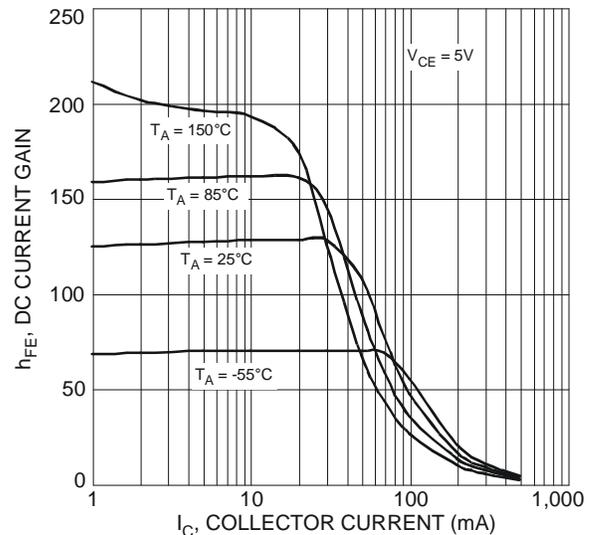
Figure 2 Typical DC Current Gain vs. Collector Current
