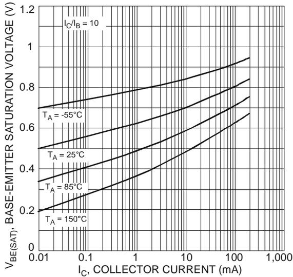
Figure 5 Typical Base-Emitter Saturation Voltage vs. Collector Current
