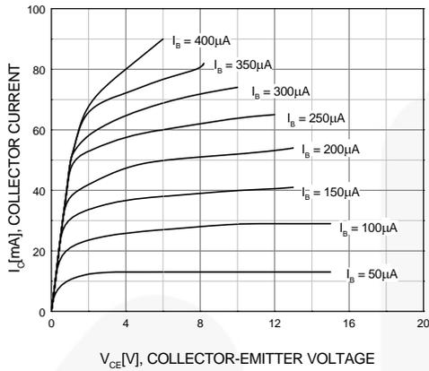
**Figure 1. Static Characteristic**
