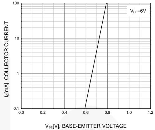
**Figure 2. Transfer Characteristic**
