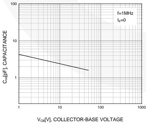
**Figure 5. Output Capacitance**
