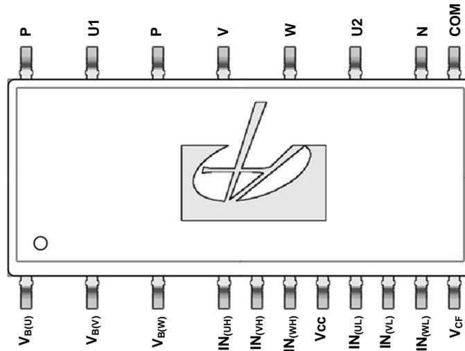
Figure 1. Pin Configuration
