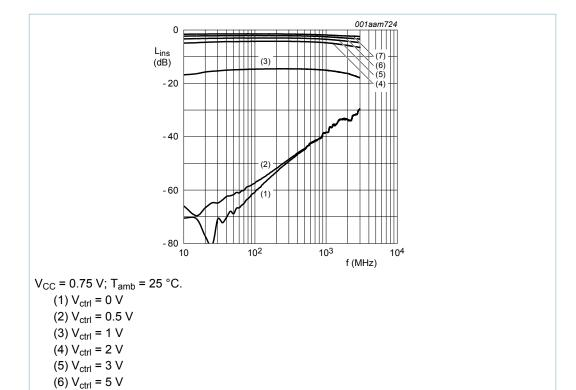
Figure 4. Insertion loss as function of frequency (typical values)
