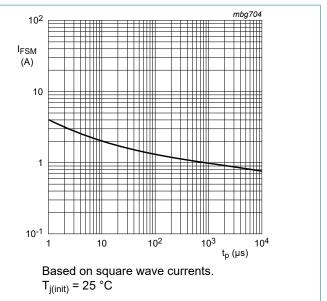
Fig. 4. Non-repetitive peak forward current as a function of pulse duration; typical values
