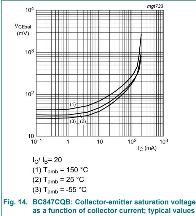
Fig. 14. BC847CQB: Collector-emitter saturation voltage as a function of collector current; typical values
