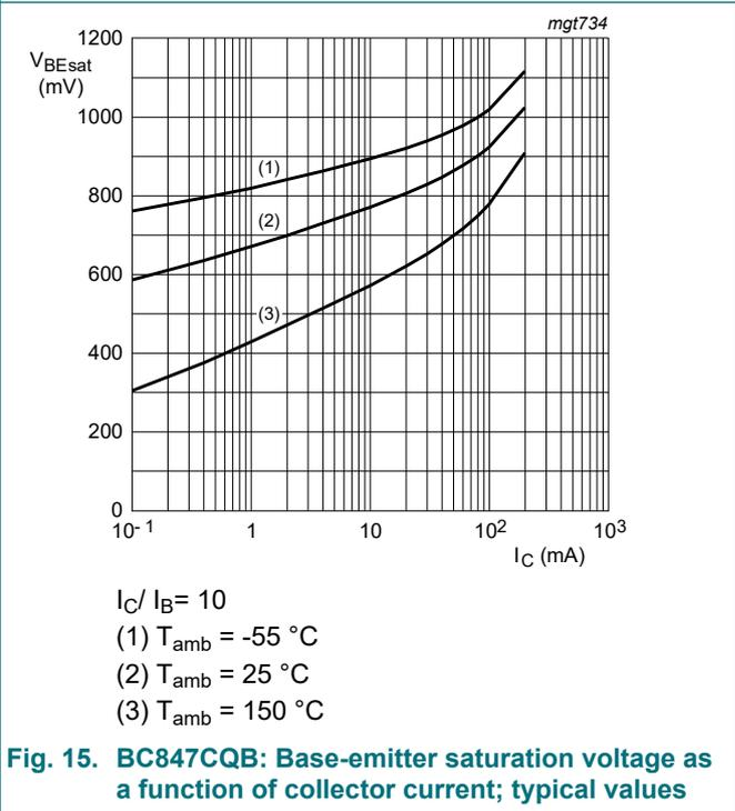
Fig. 15. BC847CQB: Base-emitter saturation voltage as a function of collector current; typical values
