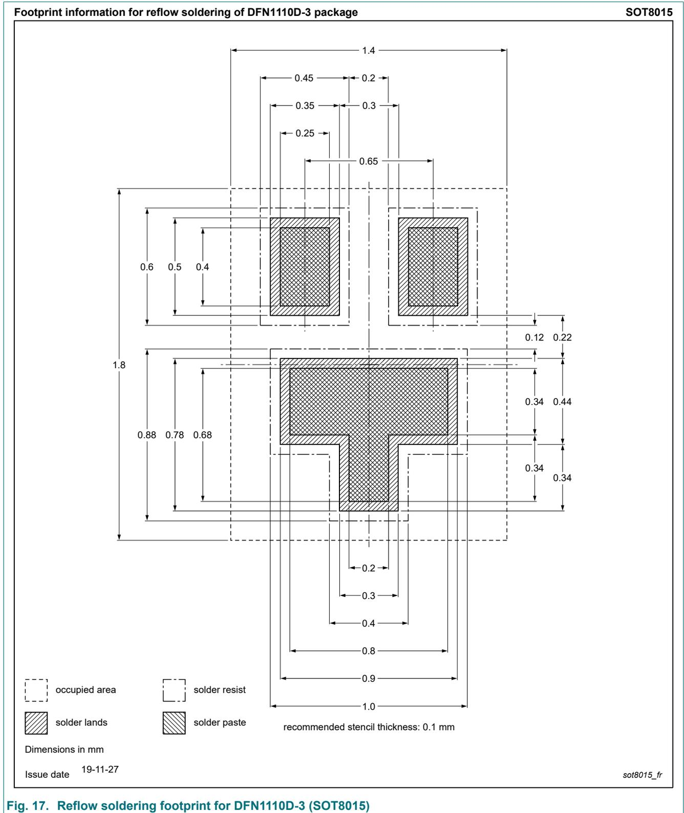
Fig. 17. Reflow soldering footprint for DFN1110D-3 (SOT8015)
