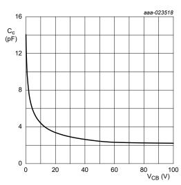
$f = 1 \text{ MHz}; T_{amb} = 25 \text{ °C}$
