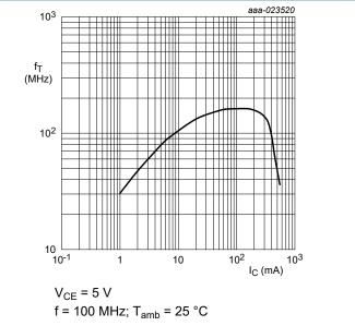
Fig. 17. Transition frequency as a function of collector current; typical values
