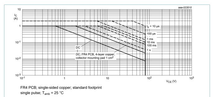
Fig. 2. Safe operating area; junction to ambient; continous and peak collector currents as a funtion of collecoremitter voltage
