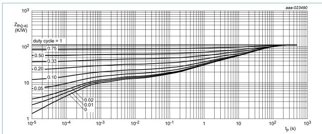
FR4 PCB; single-sided copper; tin-plated; mounting pad for collector 1 cm<sup>2</sup>
