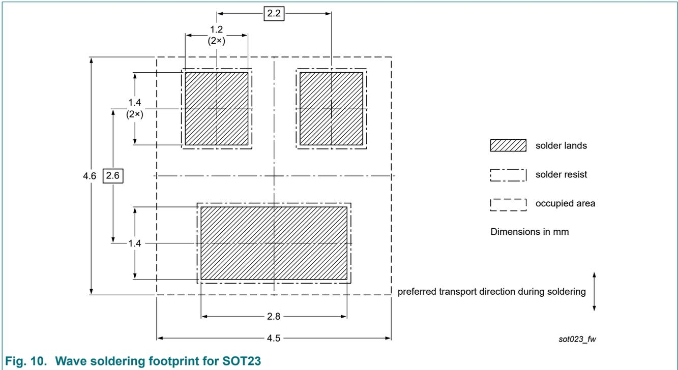
Fig. 10. Wave soldering footprint for SOT23
