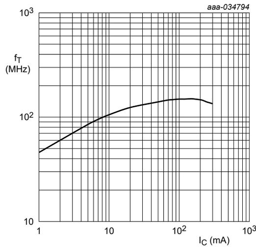
Fig. 7. Transition frequency as a function of collector current; typical values
