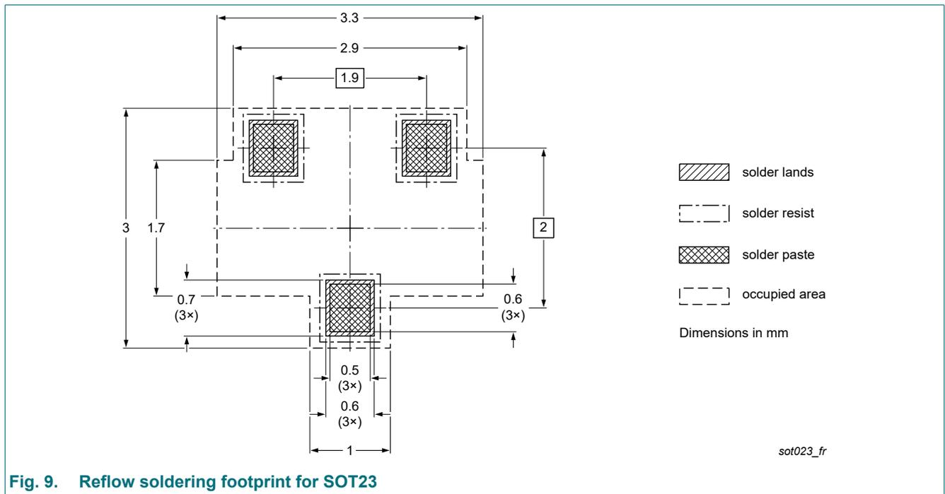
Fig. 9. Reflow soldering footprint for SOT23
