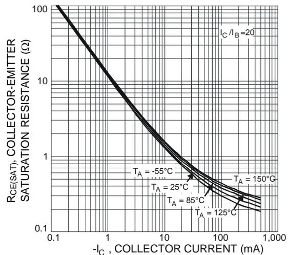
Fig. 8 Typical Collector-Emitter Saturation Resistance vs. Collector Current
