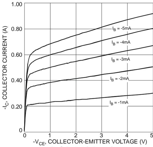
Fig. 3 Typical Collector Current vs. Collector-Emitter Voltage
