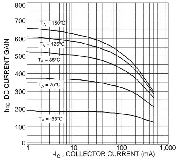
Fig. 4 Typical DC Current Gain vs. Collector Current
