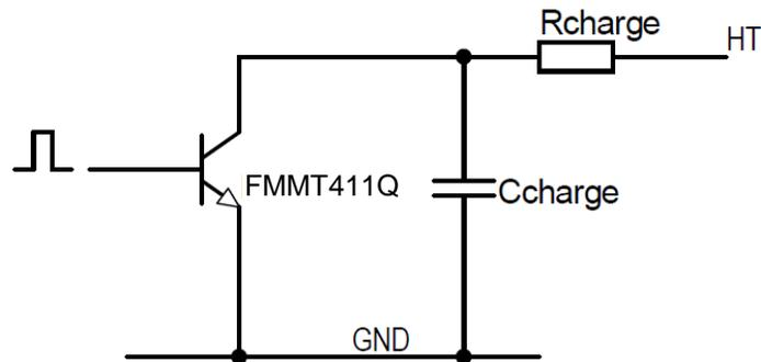
The effect of parasitic inductance in the circuit must be considered. Excessive inductance will reduce the current pulse height and slew current pulse edges. Loop area enclosed by the power circuit and track lengths should be minimized.
