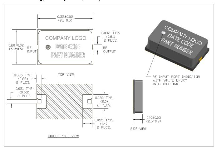
The hatched metal area on circuit side of device is RF, DC and thermal grounded.
