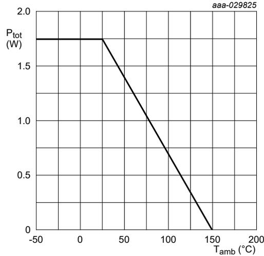
FR4 PCB, single-sided copper, tin-plated, mounting pad for collector 1 cm<sup>2</sup>.
