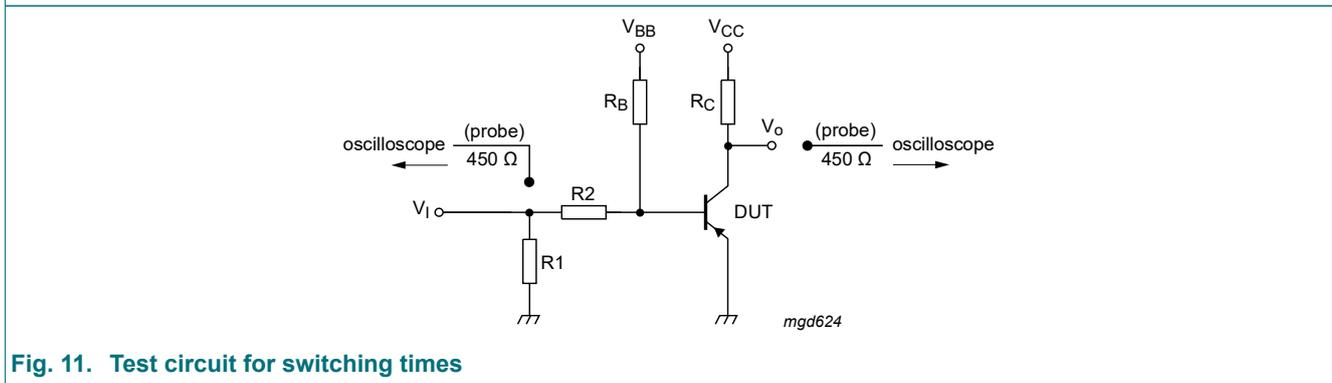
Fig. 11. Test circuit for switching times
