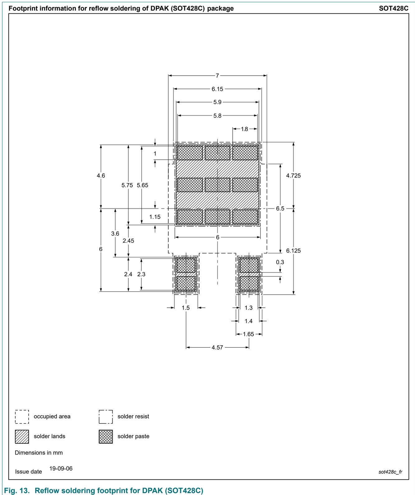
Fig. 13. Reflow soldering footprint for DPAK (SOT428C)
