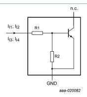
Fig. 41. TR1 (NPN): Resistor test circuit
