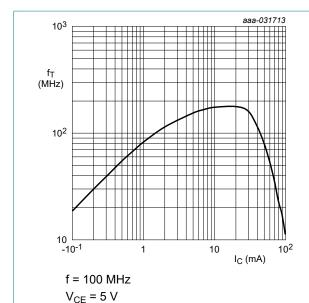
Fig. 39. TR1 (NPN): Transition frequency as a function of collector current; typical values of built-in transistor
