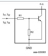
Fig. 42. TR2 (PNP): Resistor test circuit
