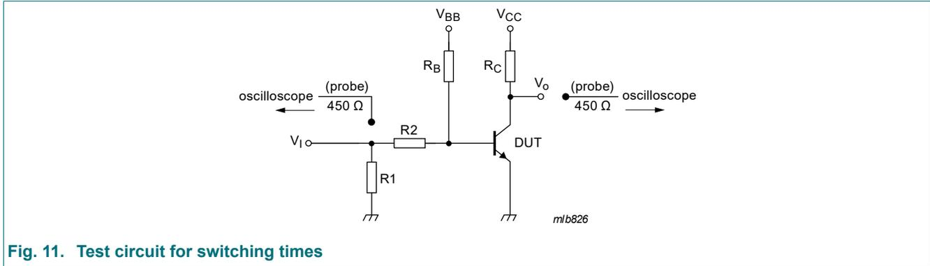
Fig. 11. Test circuit for switching times
