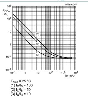
Fig. 15. Collector-emitter saturation resistance as a function of collector current; typical values
