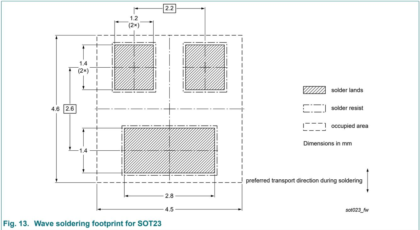
Fig. 13. Wave soldering footprint for SOT23
