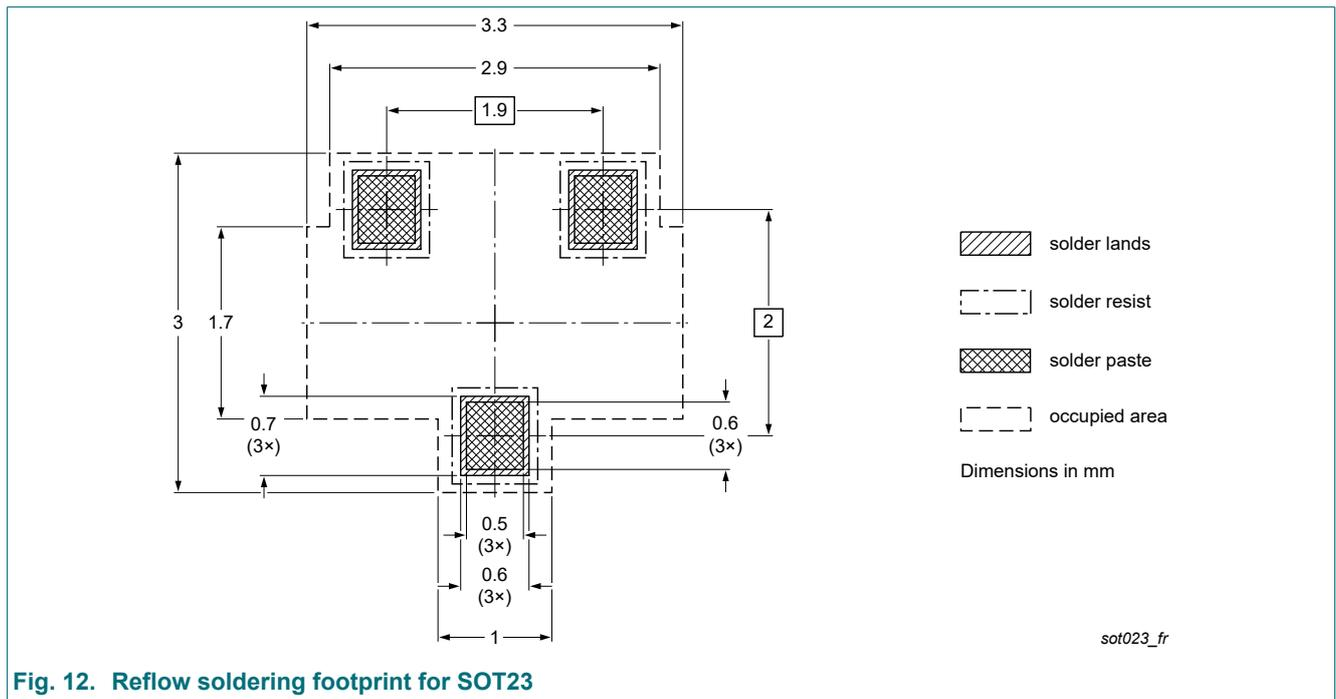
Fig. 12. Reflow soldering footprint for SOT23
