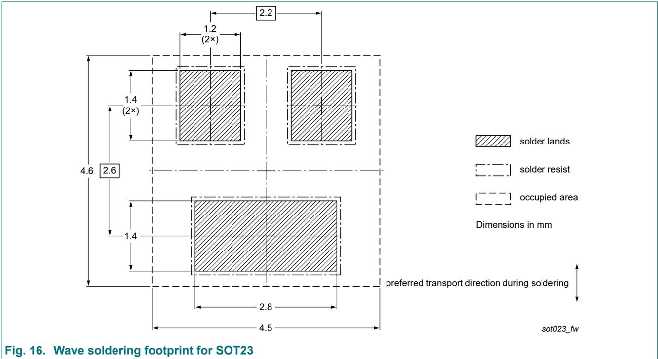
Fig. 16. Wave soldering footprint for SOT23
