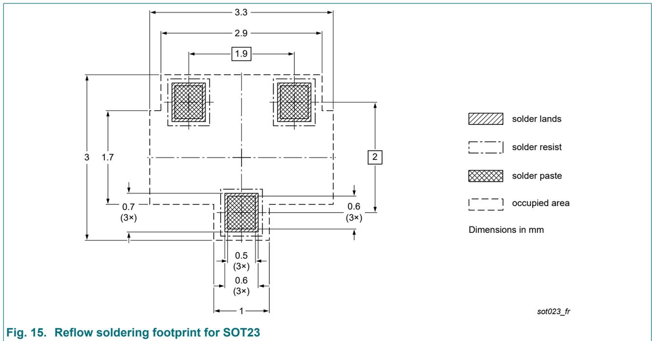
Fig. 15. Reflow soldering footprint for SOT23
