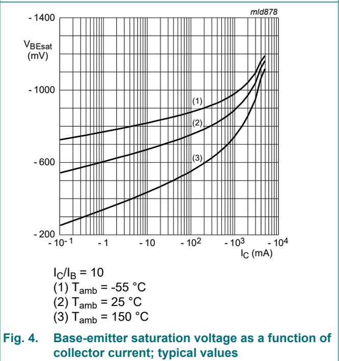
Fig. 4. Base-emitter saturation voltage as a function of collector current; typical values
