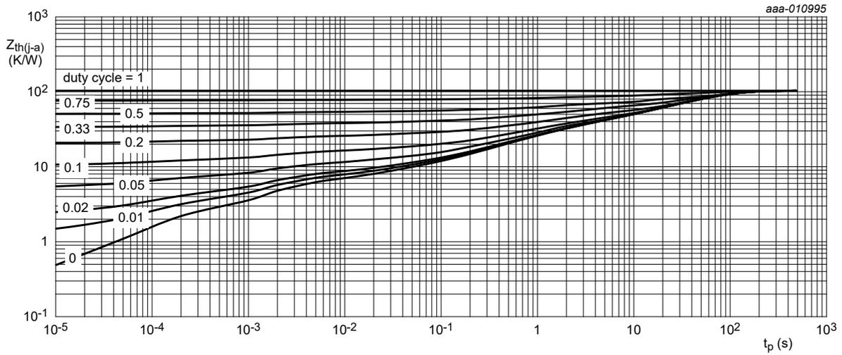
FR4 PCB, 35  $\mu$ m single-sided copper, tin-plated, mounting pad for collector 1 cm<sup>2</sup>.
