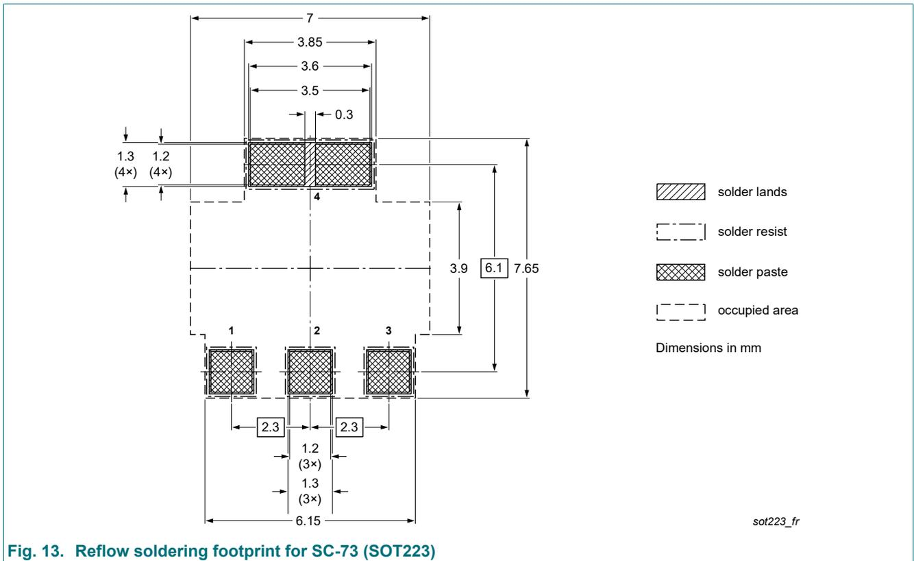
Fig. 13. Reflow soldering footprint for SC-73 (SOT223)
