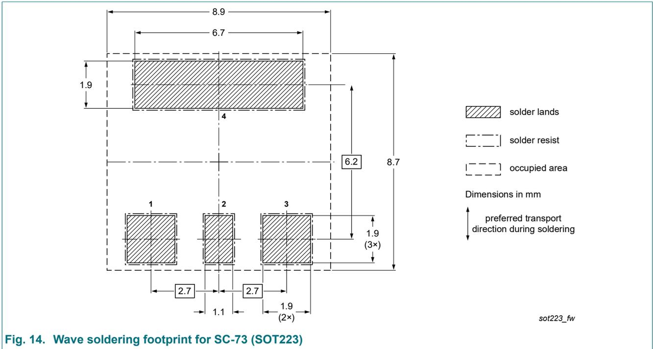
Fig. 14. Wave soldering footprint for SC-73 (SOT223)
