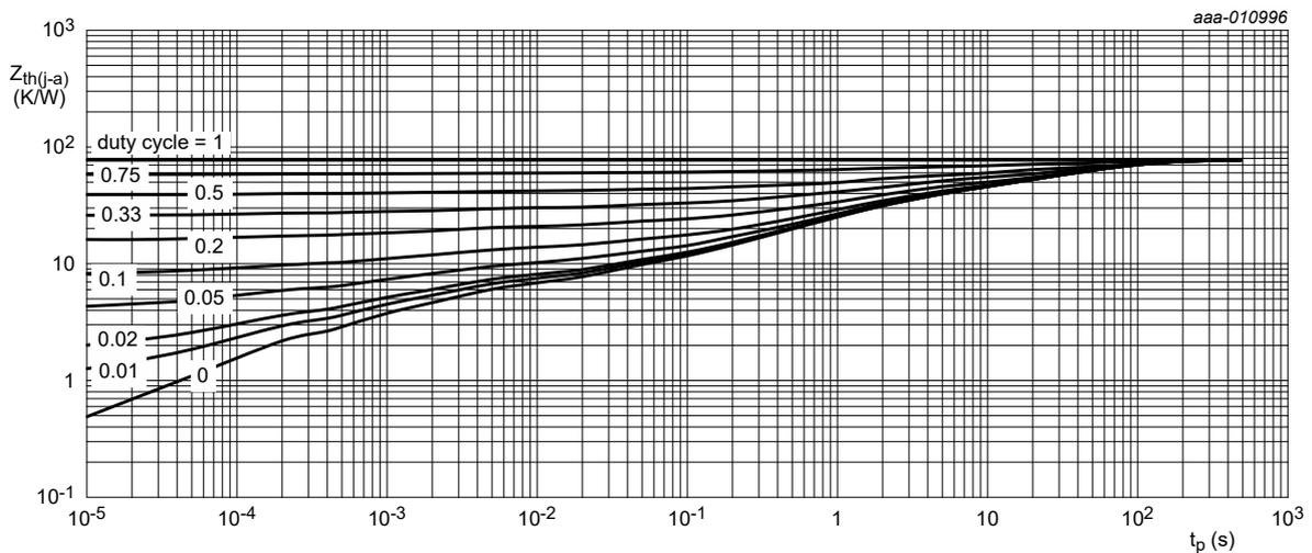
FR4 PCB, 35  $\mu$ m single-sided copper, tin-plated, mounting pad for collector 6 cm<sup>2</sup>.
