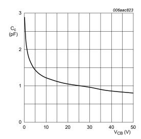
Fig. 21. PDTC143ZQC: Collector capacitance as a function of collector-base voltage; typical values
