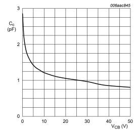
PDTC143XQC: Collector capacitance as a Fig. 9. function of collector-base voltage; typical values
