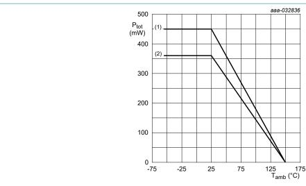
(1) FR4 PCB; single-sided; 70 µm copper; standard footprint
